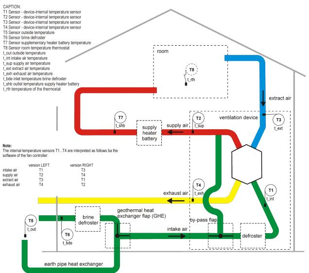
Fig. 14: General system configuration with CLIMOS F 200 Comfort series
