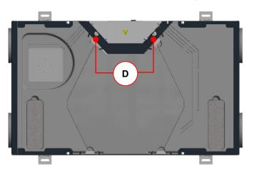
Fig. 35: Screws **D** for fixing the control casing
