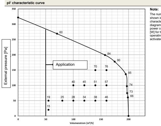
The numerical values shown in the  $p\dot{V}$  characteristic curve diagram indicate the power consumption in [W] for the respective operating points without activated defroster.
