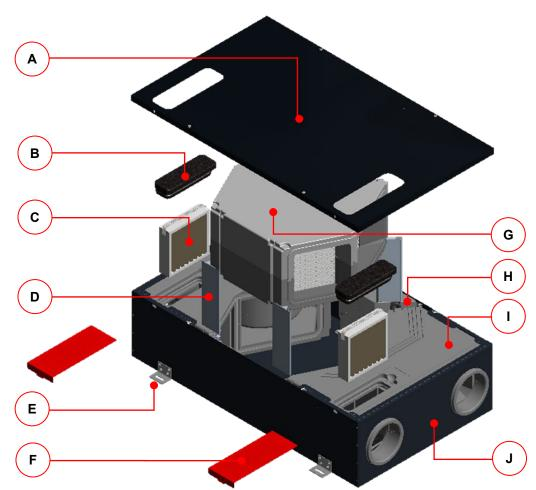
Fig. 1: Main components of the CLIMOS ventilation unit
