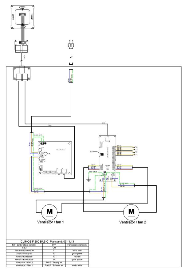
Fig. 56: Terminal assignment circuit diagram CLIMOS Basic
