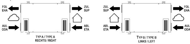
Fig. 23: Arrangement of air connections according to type R (right - type A) / L (left - type B)
