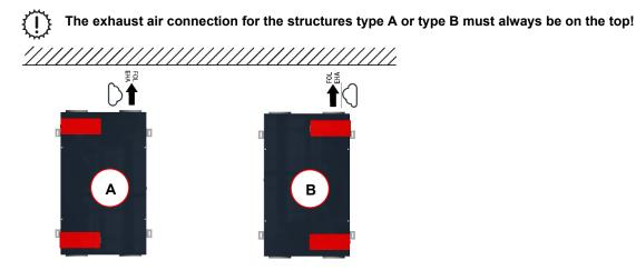
Fig. 20: Installation position mounted vertically on the wall
