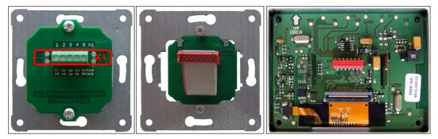
Fig. 28: Connecting board with terminal X1 on a concealed base plate; ribbon cable to the connecting board; TFT control panel board (from left to right)
