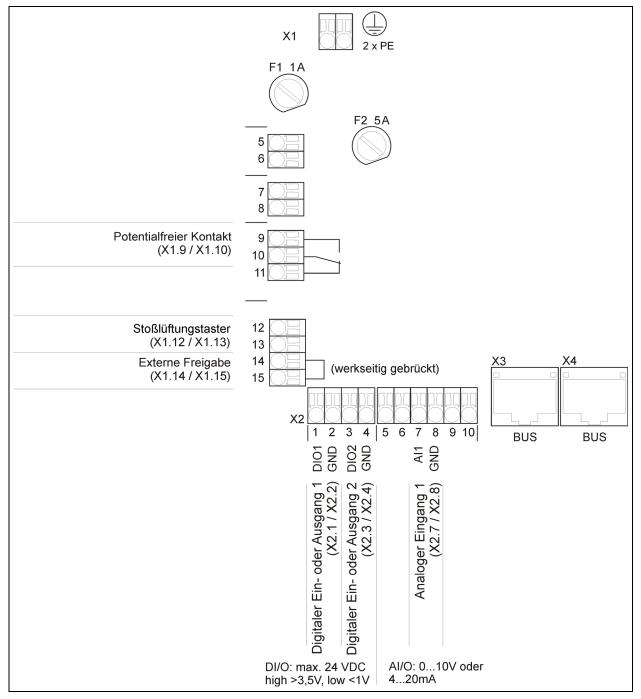
Fig. 58: Master-Controller terminal assignment
