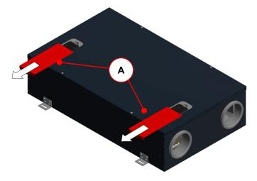
Fig. 44: Pulling out 2 design filter covers A
