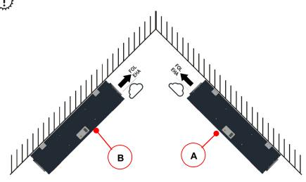
Fig. 22: Installation position mounted vertically on the wall slope
