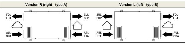
Table 40: Arrangement of air connections according to type R (right - type A) / L (left - type B)
