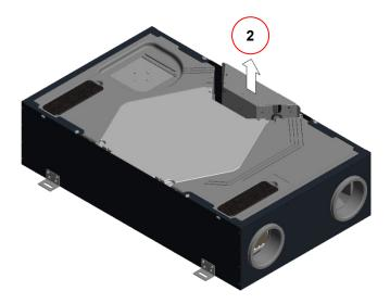
Fig. 38: Removing the control casing towards the top
