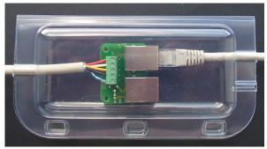
Fig. 26: Adapter circuit board
