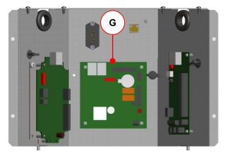
Fig. 40: Control casing with Master Controller G
