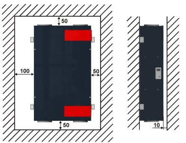
Fig. 15: Distances from adjacent surfaces in mm
