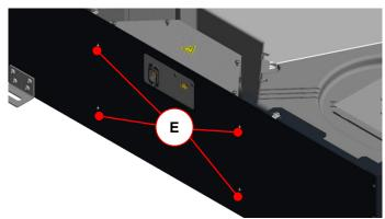
Fig. 41: Establishing the keyhole connection
