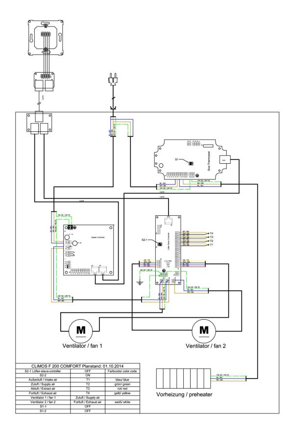
Fig. 57: Terminal assignment circuit diagram CLIMOS Comfort
